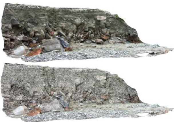
Figure 3: Image-covered mesh (above) and its wireframe (below) generated using smartphone imagery and 123D Catch (Micheletti et al. , 2014).
